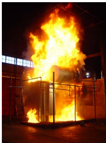
Simulated transformer fire prior to CAF application.
