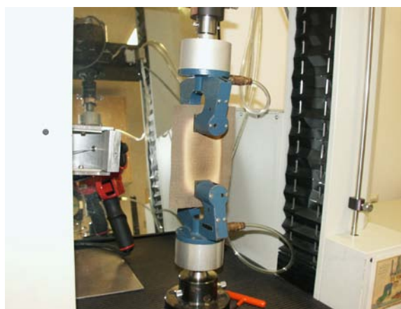
Tensile strength testing of PPE fabric.
