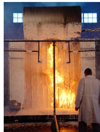
Simulated transformer fire after CAF application.
