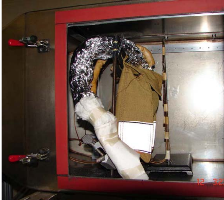
Radio inside of "pocket" from turnout gear. Radios that were protected inside the turnout gear pocket were able to operate at the Thermal Class III temperature of 260°C (500°F).
