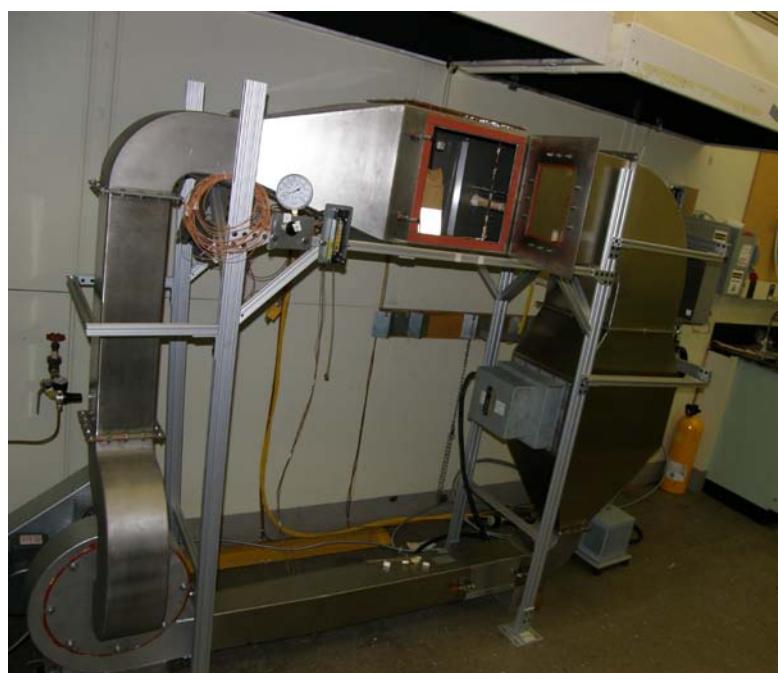
Photograph of the NIST Fire Equipment Evaluator (FEE). The test section (open area bounded by red) has radio protected by a "pocket" in place.
