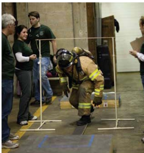
Research showed that the simple task of ducking under an obstacle appeared to be significantly more difficult while wearing PPE than while not wearing PPE, which has important implications both for safety and in affecting functional capabilities of the firefighter on the fireground, as well as any other response requiring firefighting PPE. (Photo Credit: Board of Trustees of the University of Illinois)
