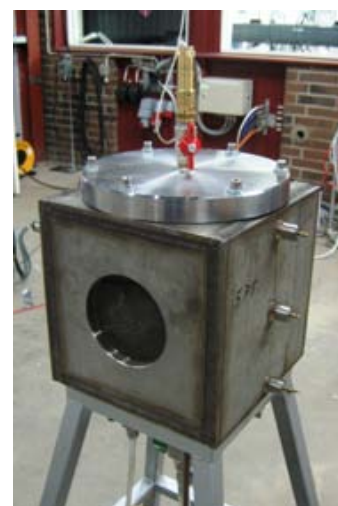
Explosion Chamber Used in Test. (Photo Credit: SP)
