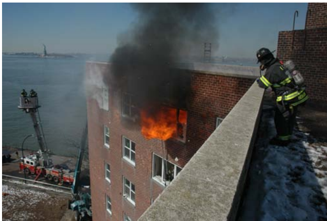
Photograph of a wind driven fire that has vented out of the living room windows. The fire started in the bedroom (two windows to the left).
